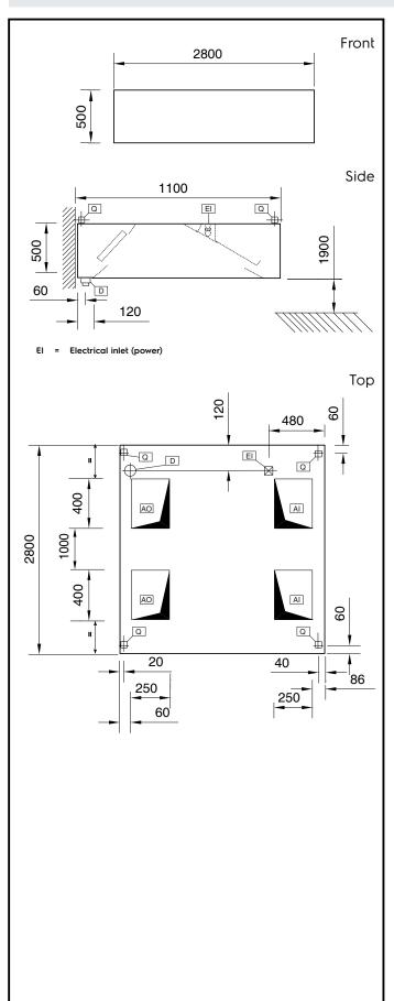
**Electric** Supply voltage: 641253 (STPF1128) 220 V/1N ph/50 Hz **Total Watts:** 0.24 kW Capacity: Supply capacity: 2580 m<sup>3</sup>/h **Key Information:** External dimensions, Width: 2800 mm External dimensions, Depth: 1100 mm 500 mm External dimensions, Height: Net weight: 176 kg Air Emission:
